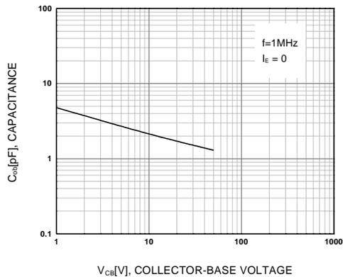
Figure 5. Output Capacitance
