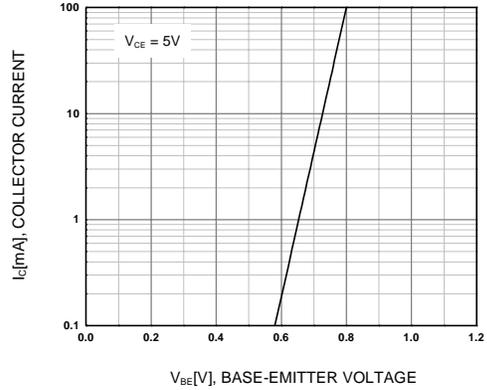
Figure 2. Transfer Characteristic
