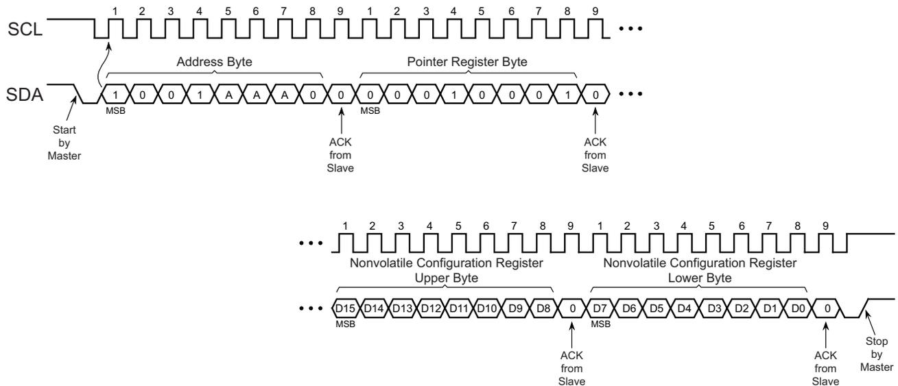
**Figure 6-7. Read from Nonvolatile Configuration Register**
