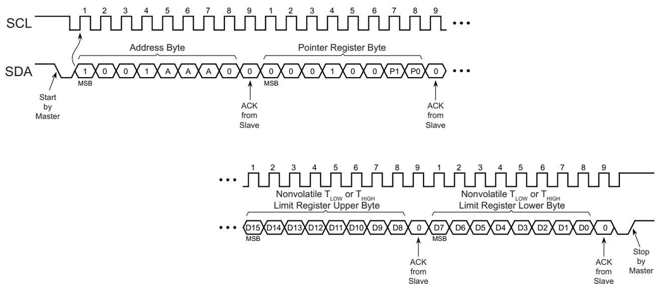
**Figure 6-11. Read to Nonvolatile T<sub>LOW</sub> or T<sub>HIGH</sub> Limit Register**
