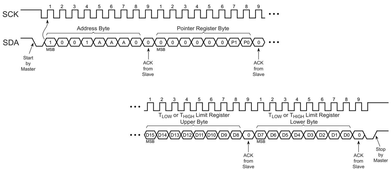
**Figure 6-9. Read from  $T_{LOW}$  or  $T_{HIGH}$  Limit Register**
