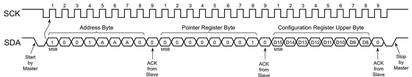
**Figure 6-5. Read from Configuration Register**
