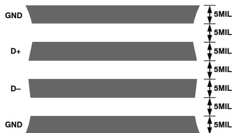
**Figure 16. Arrangements of Signal Tracks**
