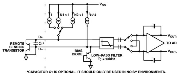
**Figure 14. Signal Conditioning for Remote Diode Temperature Sensors**
