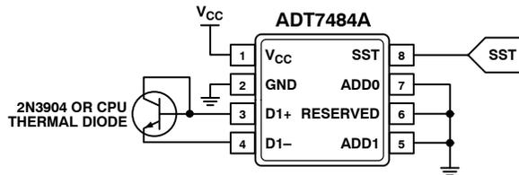
Figure 17. ADT7484A Typical Application Schematic
