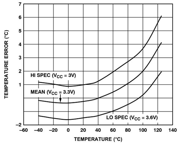
Figure 7. Remote Temperature Error
