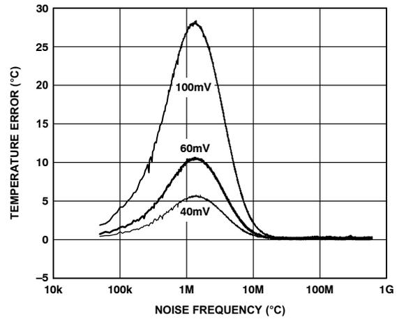
Figure 9. Temperature Error vs. Common-Mode Noise Frequency
