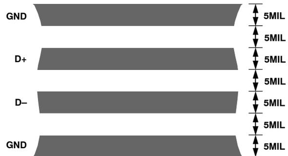
Figure 21. Typical Arrangement of Signal Tracks
