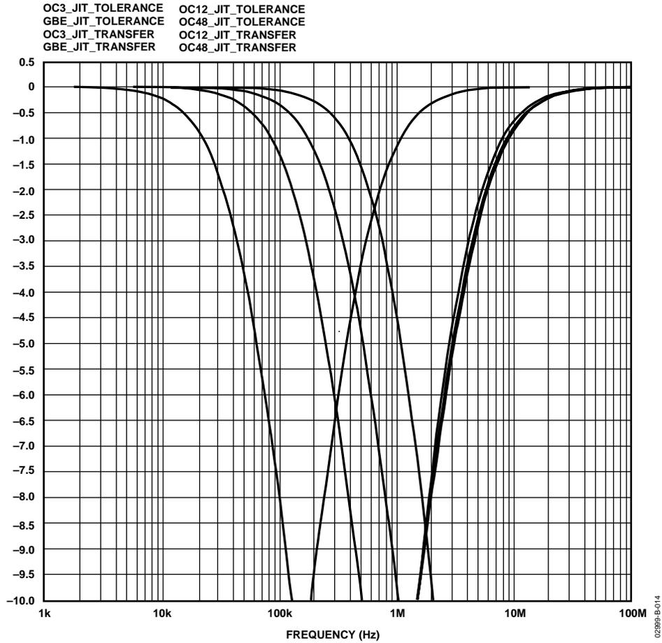
Figure 14. Jitter Transfer and Jitter Tracking Bandwidth
