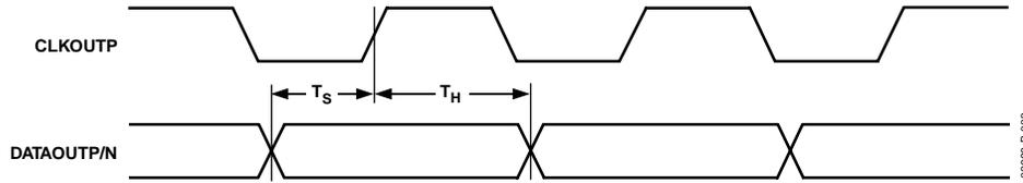
Figure 3. Output Timing
