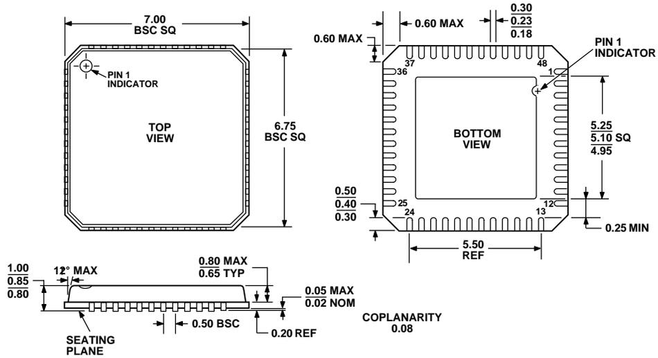
Figure 27. 48-Lead Lead Frame Chip Scale Package [LFCS]
