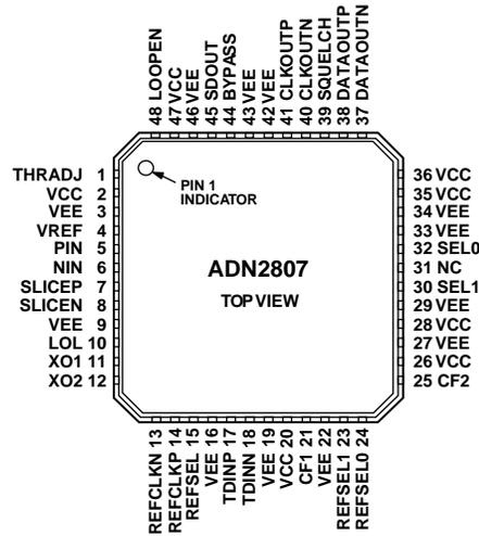
Figure 2. Pin Configuration
