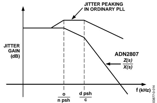
Figure 14. Jitter Response vs. Conventional PLL
