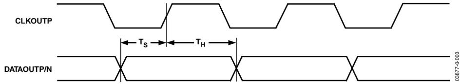
Figure 3. Output Timing
