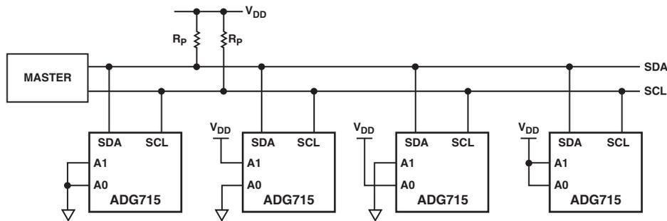
Figure 6. Multiple ADG715s On One Bus
