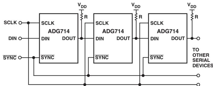
Figure 7. Multiple ADG714 Devices in a Daisy-Chained Configuration
