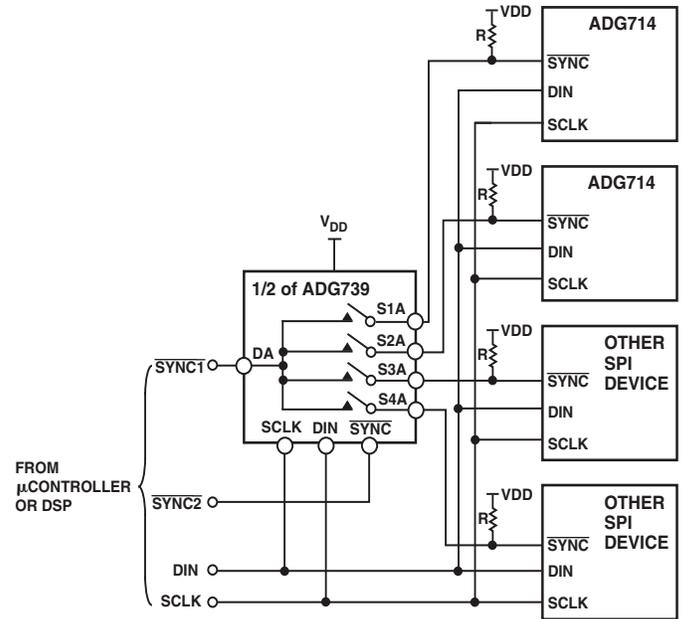
Figure 8. Addressing Multiple ADG714s Using an ADG739
