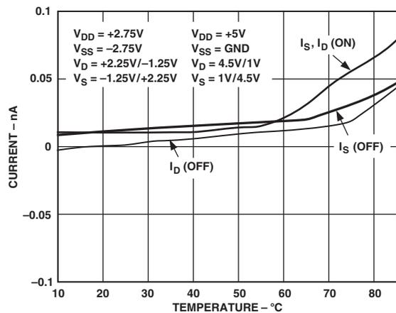
TPC 9. Leakage Currents as Function of Temperature
