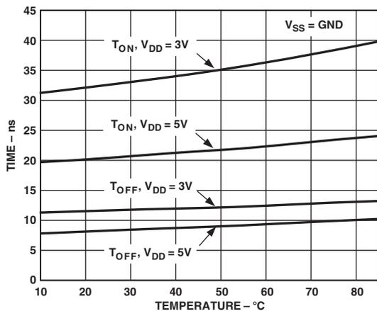
TPC 15.  $T_{ON}/T_{OFF}$  Times vs. Temperature for ADG714
