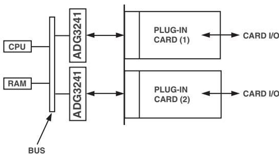
Figure 12. ADG3241 in a Hot Plug Application
