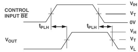
Figure 2. Propagation Delay
