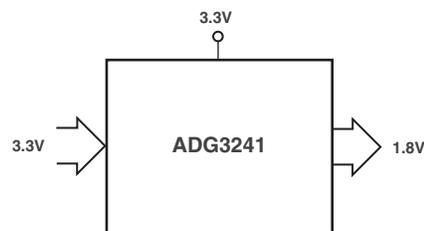
Figure 9. 3.3 V to 1.8 V Voltage Translation,  $\overline{SEL} = 0$  V
