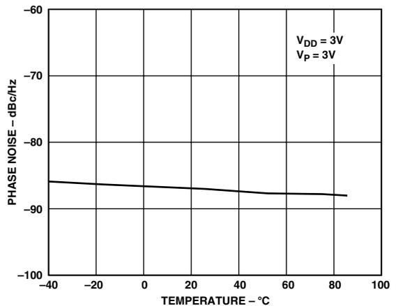
TPC 9. ADF4218 RF Integrated Phase Noise (1750 MHz, 30 kHz, 3 kHz)
