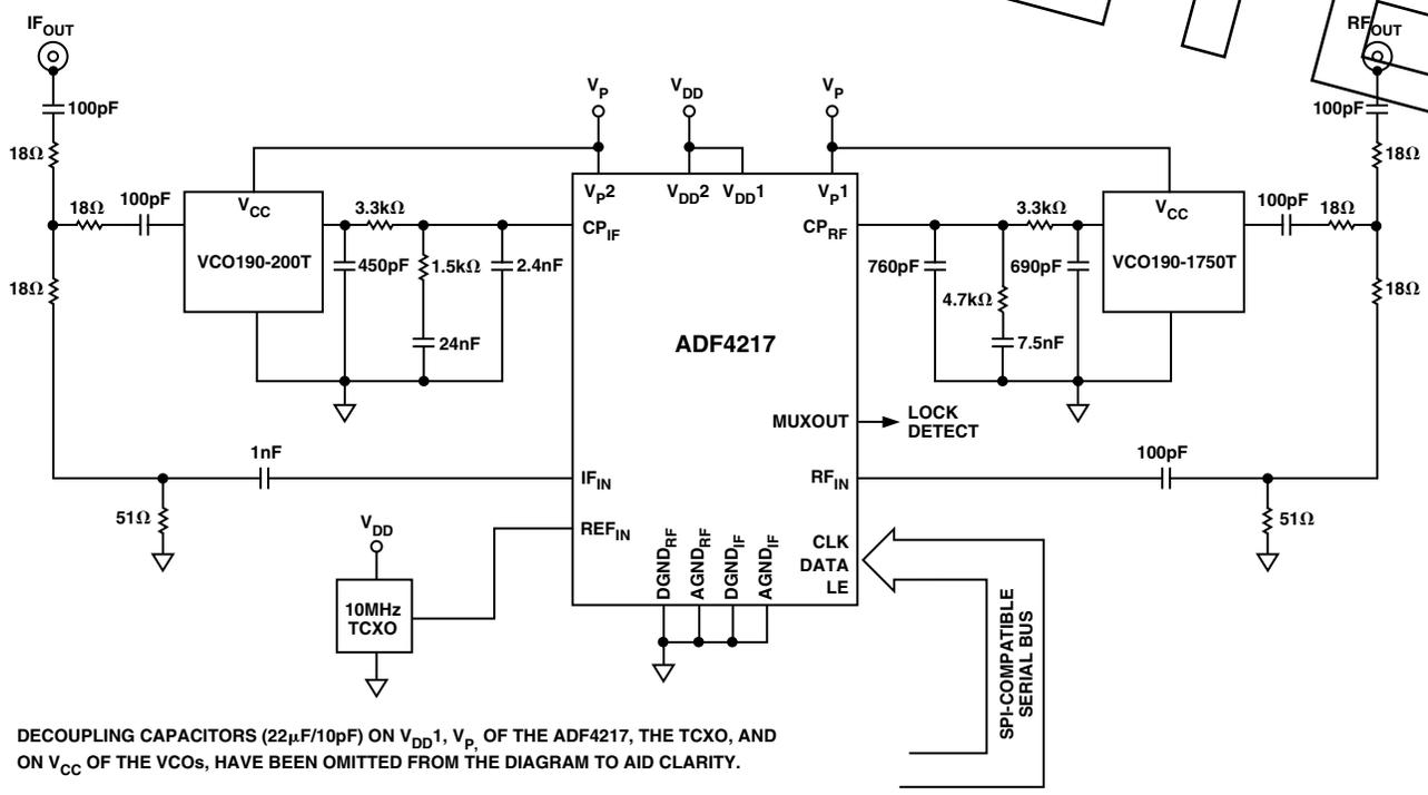
DECOUPLING CAPACITORS (22 $\mu$ F/10pF) ON  $V_{DD1}$ ,  $V_p$  OF THE ADF4217, THE TCXO, AND ON  $V_{CC}$  OF THE VCOs, HAVE BEEN OMITTED FROM THE DIAGRAM TO AID CLARITY.
