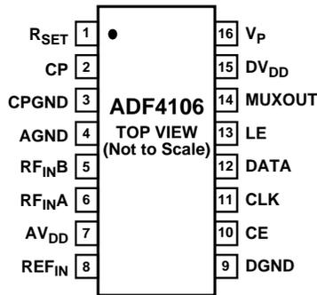
NOTE: TRANSISTOR COUNT 6425 (CMOS), 303 (BIPOLAR).
