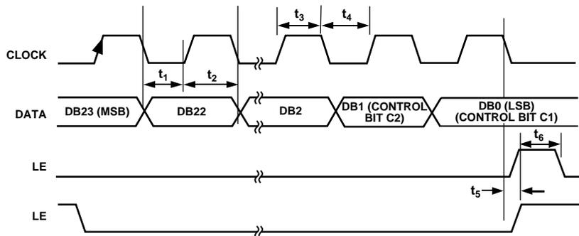
Figure 2. Timing Diagram
