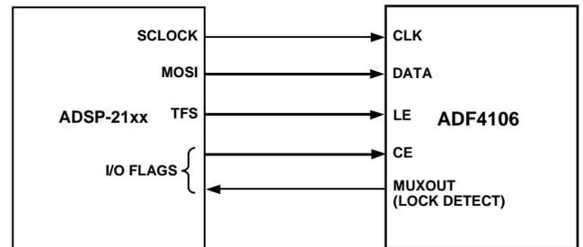
Figure 24. ADSP-21xx-to-ADF4106 Interface
