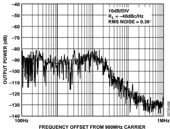
Figure 8. Integrated Phase Noise (900 MHz, 200 kHz, and 20 kHz)
