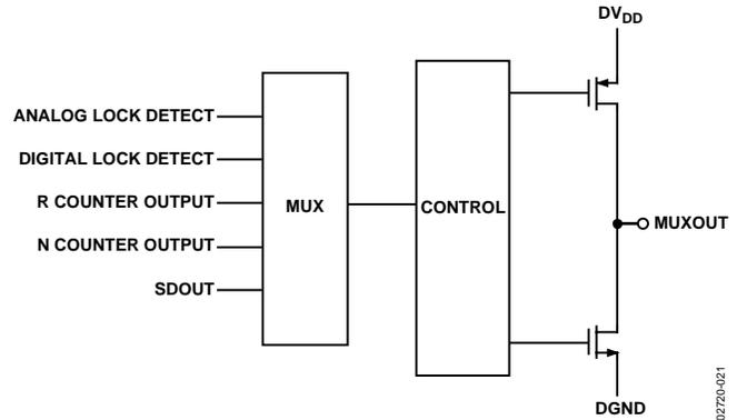
Figure 21. MUXOUT Circuit
