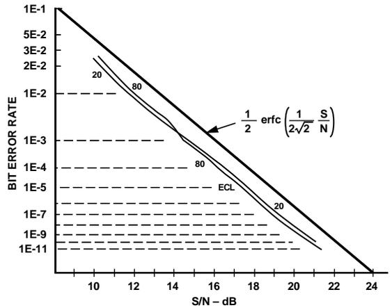
Figure 8. AD800-45 Bit Error Rate vs. Input Jitter
