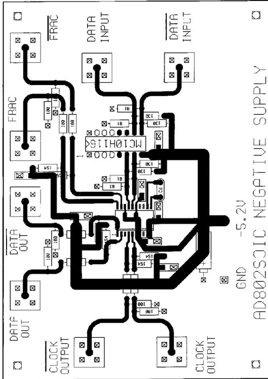
Figure 27. Negative Supply Configuration: Component Side (Top Layer)
