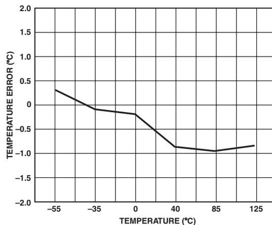
Figure 6. Typical Temperature Error @ 2.65 V
