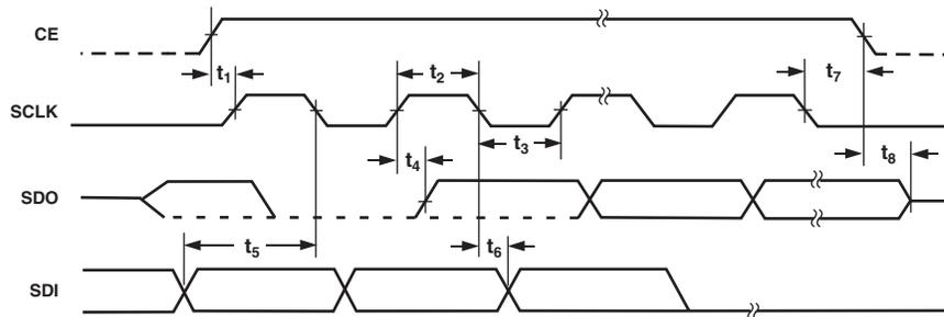
Figure 1. Timing Diagram
