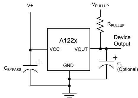
Figure 3. Typical 3-wire application circuit
