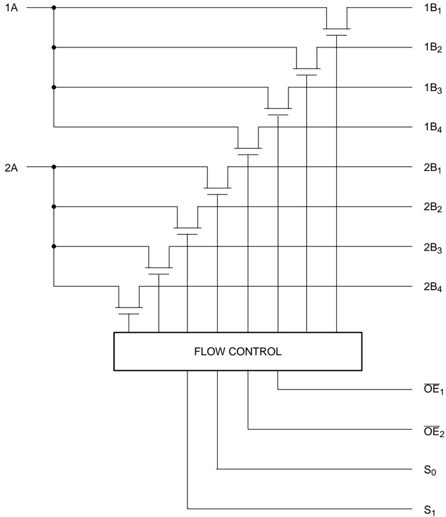
Figure 3. Logic Diagram
