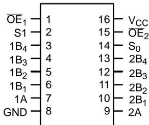
Figure 1. 16-Lead Pinout
