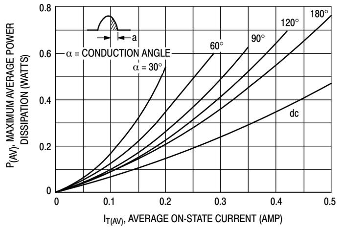
Figure 5. Power Dissipation
