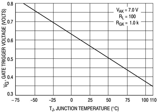
Figure 7. Typical Gate Trigger Voltage
