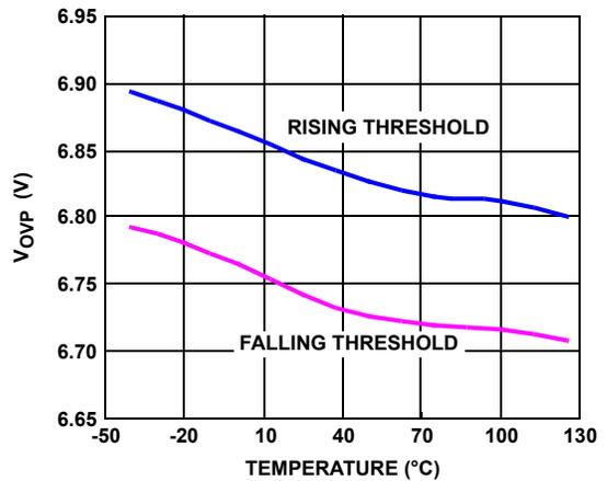
FIGURE 13. INPUT OVERVOLTAGE PROTECTION THRESHOLDS vs TEMPERATURE
