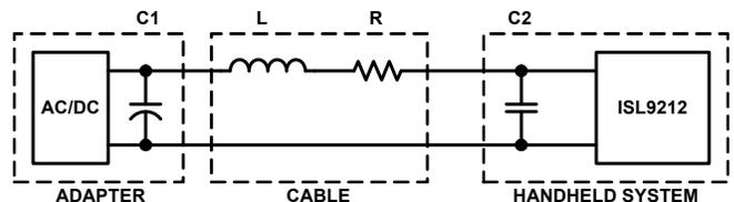
FIGURE 25. EQUIVALENT CIRCUIT FOR THE ISL9212B INPUT
