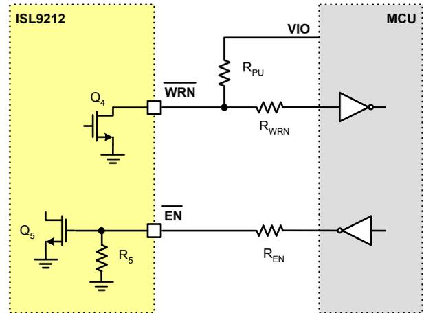
FIGURE 24. DIGITAL SIGNAL INTERFACE BETWEEN ISL9212B AND MCU
