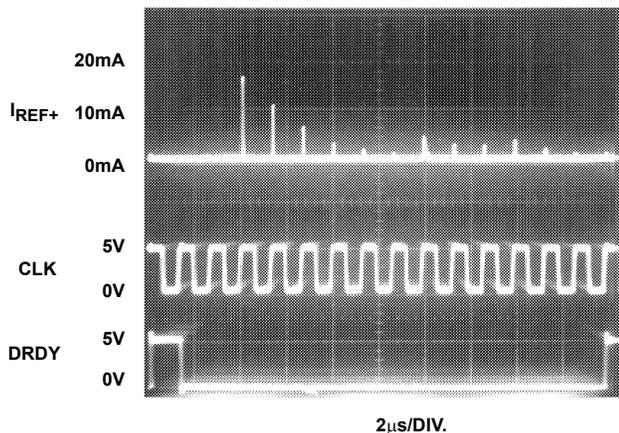
CONDITIONS: V<sub>DD</sub> = V<sub>AA+</sub> = 5.0V, V<sub>REF+</sub> = 4.608V, V<sub>IN</sub> = 2.3V, CLK = 750kHz, T<sub>A</sub> = 25°C
