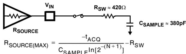
FIGURE 19. ANALOG INPUT MODEL IN TRACK MODE
