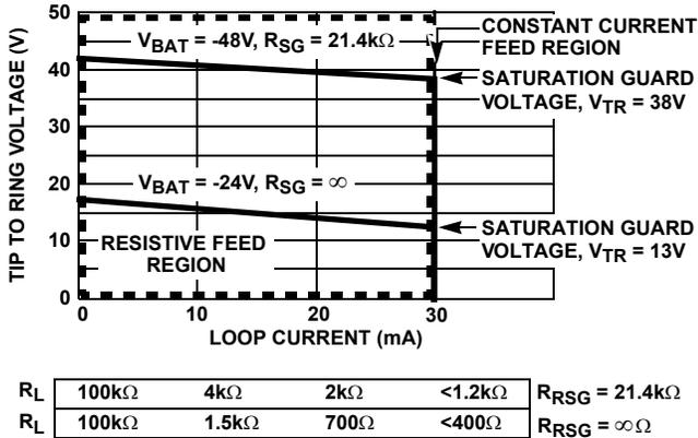
FIGURE 15. V<sub>TR</sub> vs I<sub>L</sub> AND R<sub>L</sub>
