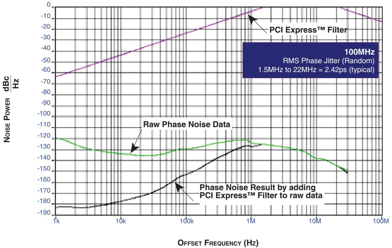
The illustrated phase noise plot was taken using a low phase noise signal generator, the noise floor of the signal generator is less than that of the device under test.
