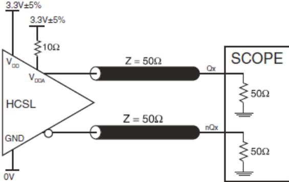
3.3V HCSL OUTPUT LOAD AC TEST CIRCUIT
