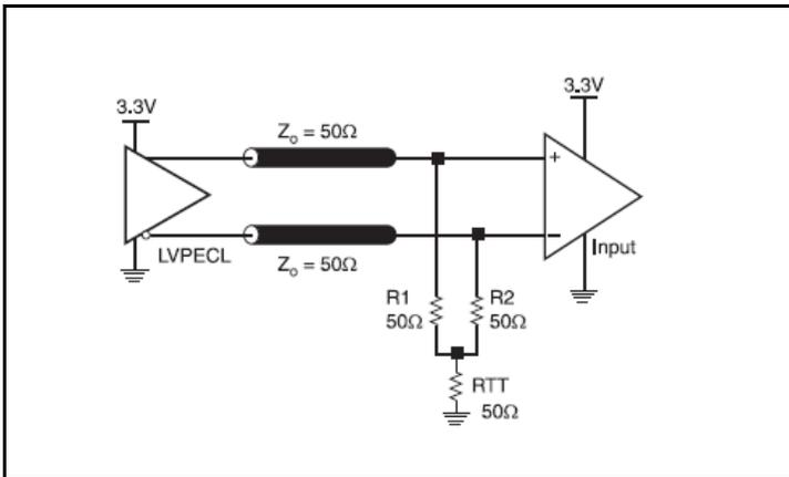
Figure 3A. Figure 4A. 3.3V LVPECL Output Termination
