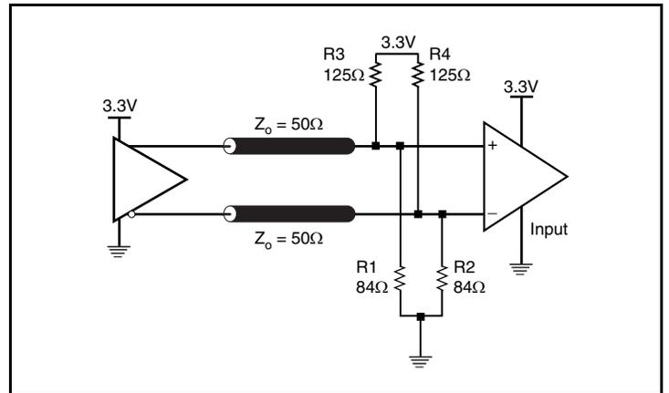
Figure 3B. Figure 4B. 3.3V LVPECL Output Termination
