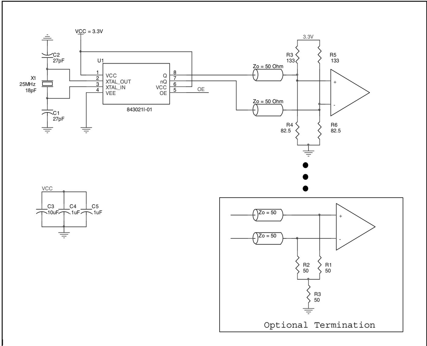
Figure 5. 8430211-01 Schematic Example
