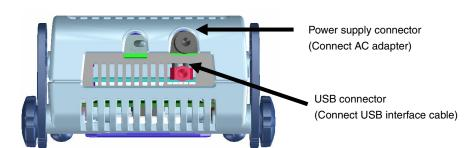
Figure 2-9. Connector Positions
