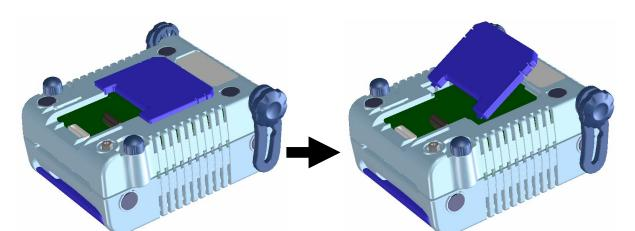
Figure 2-2. Acrylic Board Removal Method
