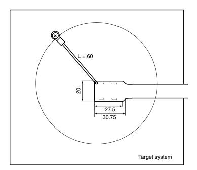
Figure 2-7. Where GND Wire Can Be Connected
