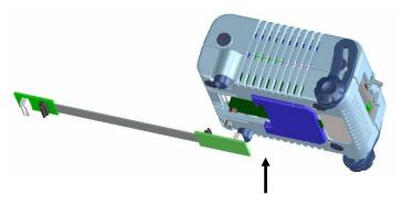
Insert CN1 and CN2 of the probe into TCN1 and TCN2 of the QB-78K0KX2.
