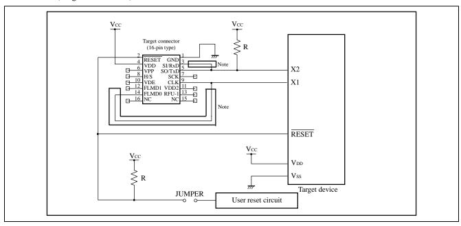
Figure 8.2 Circuit Example for 78K0S (Single-wire UART)
