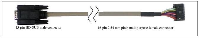
Figure 7.10 Target Cable (16-pin type) Outline
