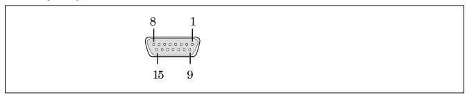
Figure 5.1 Remote Connector (D-SUB 15 pin connector (female)) Pin Assignment
