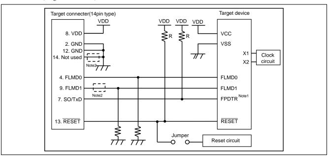
Figure 8.6 Circuit Example for V850E2 (Single-wire UART)
