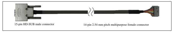
Figure 7.13 Target Cable (14-pin type) Outline
