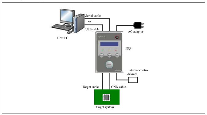
Figure 2.1 FP5 System Configuration
