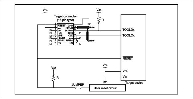
Figure 8.5 Circuit Example for 78K0 (TOOLCx, TOOLDx)
