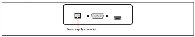
Figure 7.1 Power Supply Connector <FP5 Host Interface Side>
