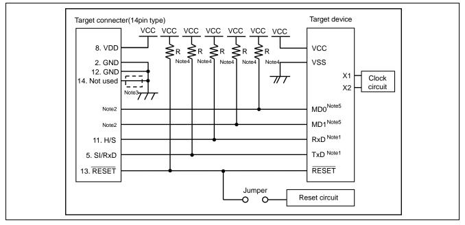
Figure 8.10 Circuit Example for RX Family and SuperH Family (Circuit Example for RX62T)
