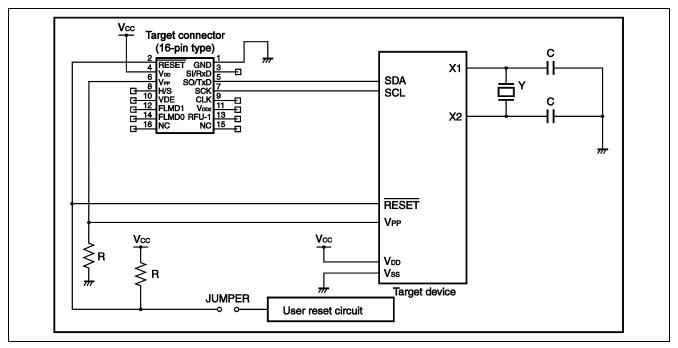
Figure 8.4 Circuit Example for I<sup>2</sup>C
