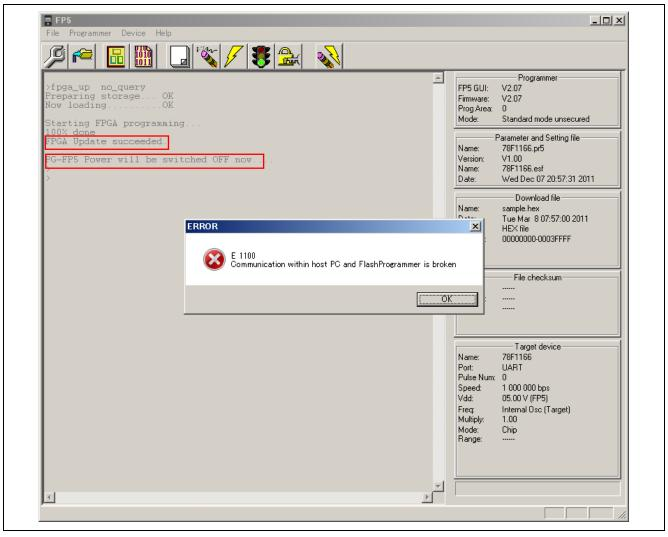
Figure 3.8 Action Log Window When FPGA Update Is Finished
