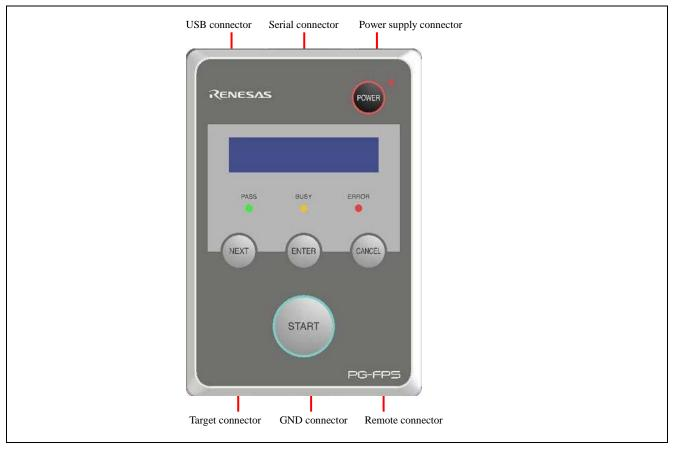
Figure 2.3 FP5 Top View < Connector>
