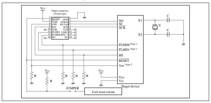
Figure 8.1 SIO-H/S Interface Circuit Example
