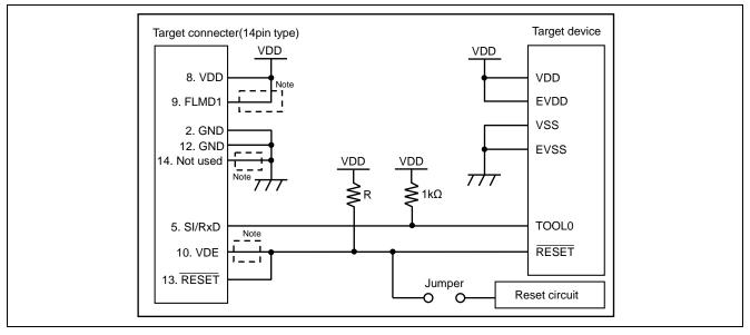
Figure 8.8 Circuit Example for RL78 Family (VDD = EVDD)
