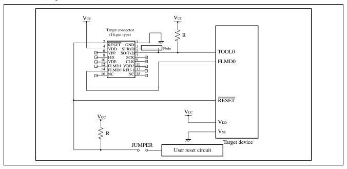
Figure 8.3 Circuit Example for 78K0R (Single-wire UART)
