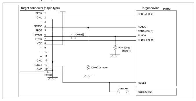
Figure 8.15 Circuit Example for RH850 family (CSI)
