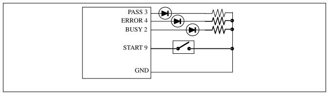
Figure 5.3 External Switch and LED Connection Example
