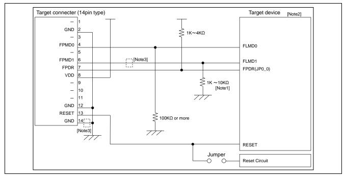
Figure 8.13 Circuit Example for RH850 family (1 wire UART)
