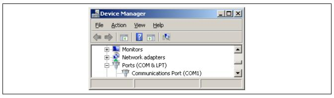
Figure 6.2 Checking the COM Port Number Settings
