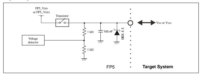
Figure 9.5  $V_{DD}$  and  $V_{DD2}$  Pins
