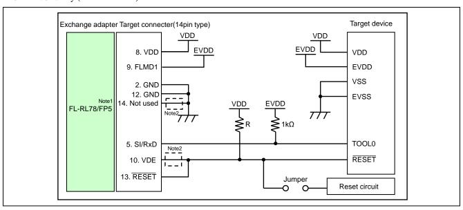
Figure 8.9 Circuit Example for RL78 Family (VDD  $\neq$  EVDD)
