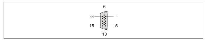
Figure 7.11 15-Pin HD-SUB Male Connector Pin Assignment of Target Cable (16-pin type)
