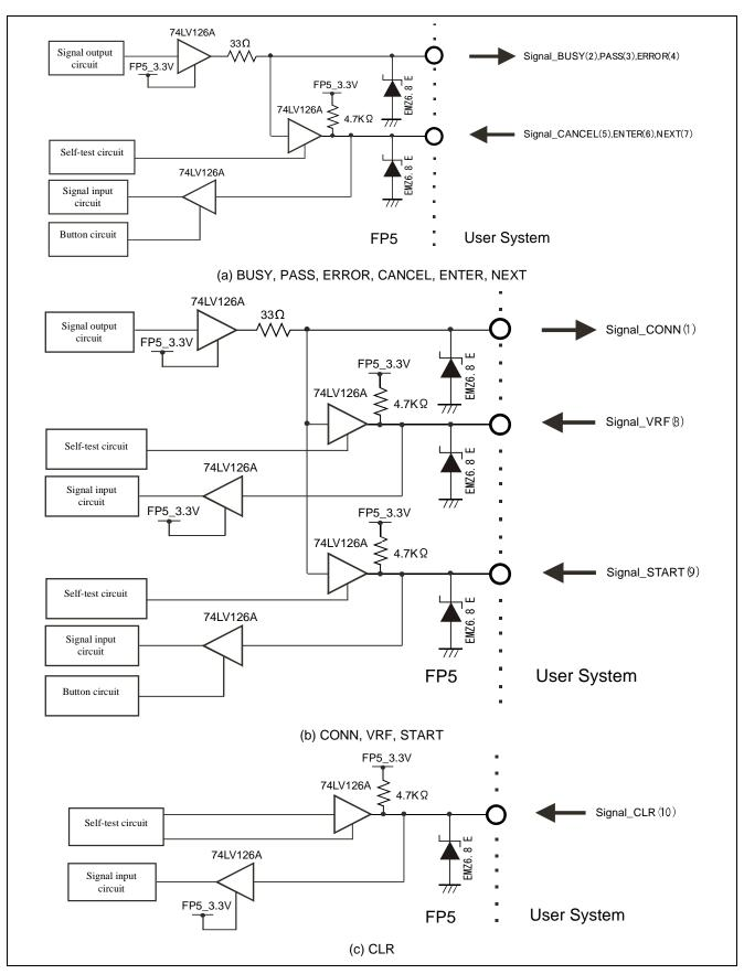
Figure 5.2 Equivalence Circuit
