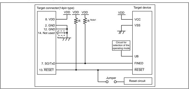
Figure 8.12 Circuit Example for RX100, RX200 series (FINE)
