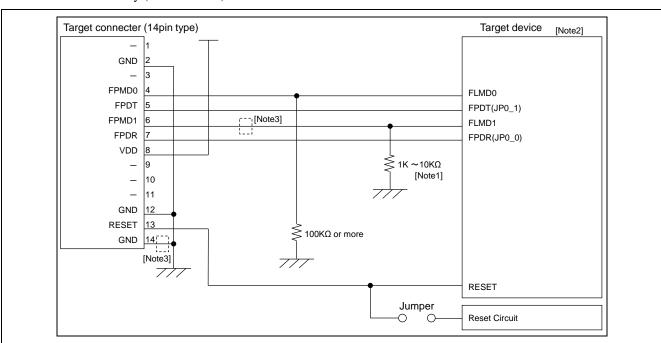
Figure 8.14 Circuit Example for RH850 family (2 wire UART)
