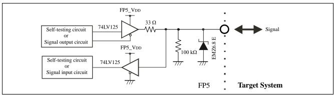
Figure 9.2 SI/RxD/FPDT and H/S Pins
