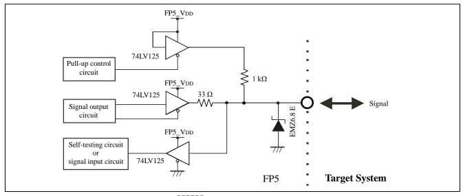
Figure 9.1 SO/TxD/IO3/FPDR/FPMD3, RESETand SCK/IO4/FPCK/FPMD4 Pins
