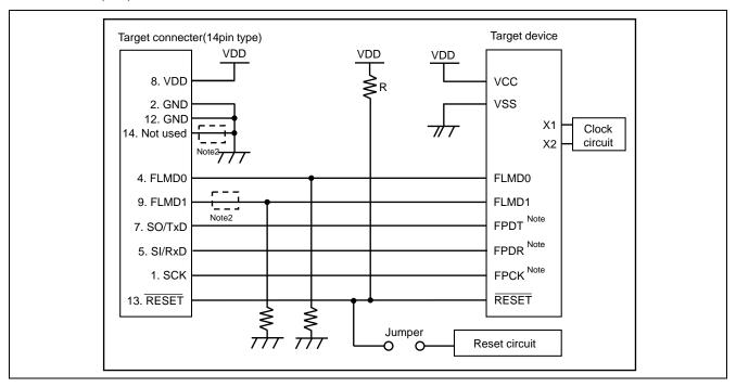
Figure 8.7 Circuit Example for V850E2 (CSI)
