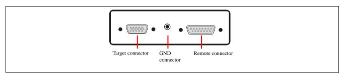
Figure 2.5 FP5 Target Connector Side
