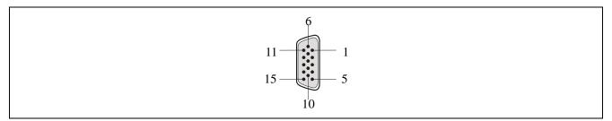
Figure 7.14 15-Pin HD-SUB Male Connector Pin Assignment of Target Cable (14-pin type)
