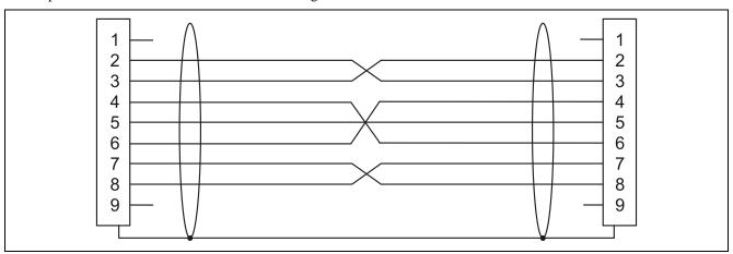
Figure 7.5 Serial Cable Connection
