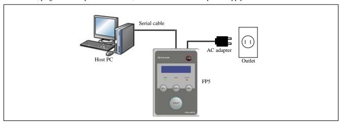
Figure 6.1 System Connections
