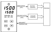
The TCU has dual outputs for providing heating and cooling to those processes that require them. Many extruder applications require both heating and cooling to maintain accurate extruder barrel and die temperatures. The TCU is easily configured for these applications.
