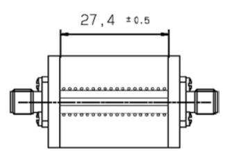
Inputs/Outputs of the calibration board and test fixture are equipped with SMA type receptacle connectors, RADIALL part number R125 510 000. The length of the RF tracks are the same on the calibration board and the test fixture circuits. The insertion loss of the relay itself is calculated by subtracting the insertion loss of the "calibration board" to the insertion loss of the "relay welded on the test fixture".
