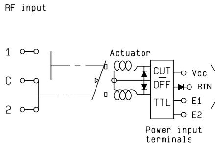
**WITH CUT-OFF, TTL AND INDICATOR CONTACT**
