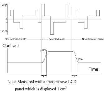
$V_{LCD}$ : Operating voltage  $f_{FRM}$ : Frame frequency  $t_r$ : Response time (rise)  $t_f$ : Response time (fall)
