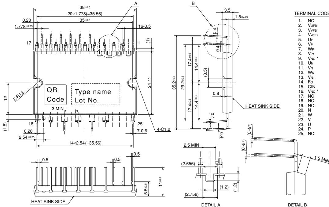
\*) Two VNC terminals (9 & 16 pin) are connected inside DIP-IPM, please connect either one to the 15V power supply GND outside and leave another one open.
