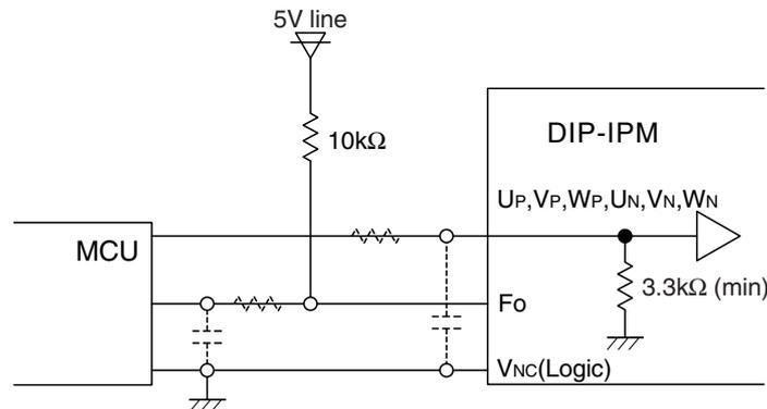
**Note :** The setting of RC coupling at each input (parts shown dotted) depends on the PWM control scheme and the wiring impedance of the printed circuit board.
