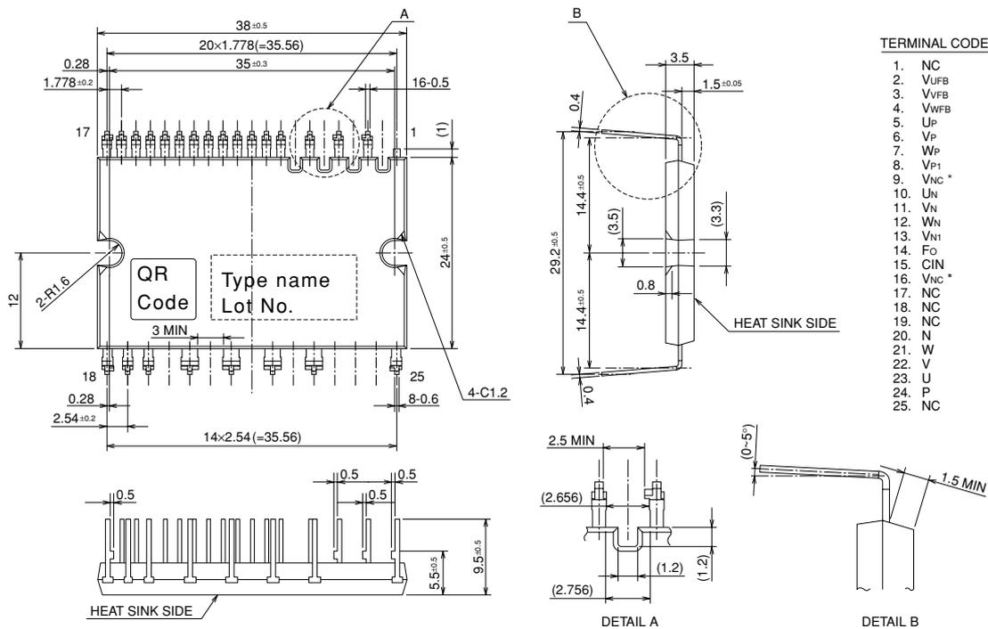
\*) Two V<sub>NC</sub> terminals (9 & 16 pin) are connected inside DIP-IPM, please connect either one to the 15V power supply GND outside and leave another one open.
