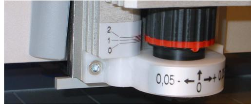
Figure 16 Depth adjuster
