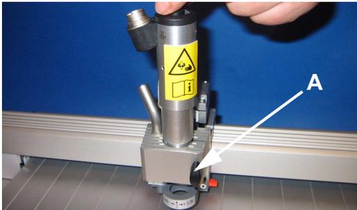
Figure 5 Inserting the engraving spindle
