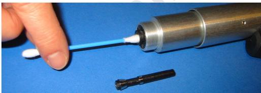
Figure 23 Cleaning the collet chuck of the engraving spindle
