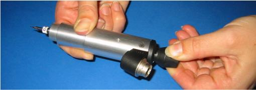
Figure 18 Loosening the engraving spindle
