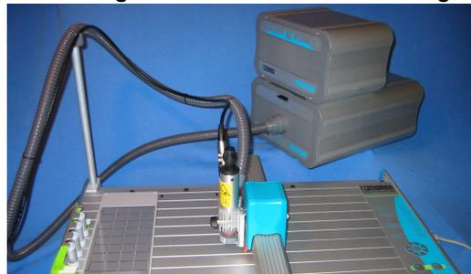
Figure 9 Connections to the engraving head
