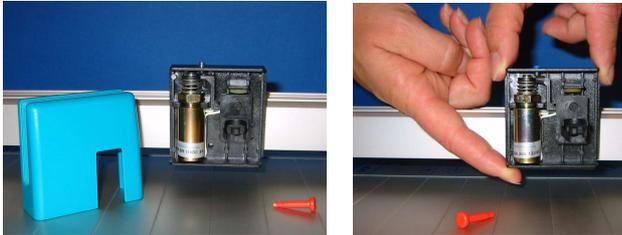
Figure 1 Removing the pen lowering unit
