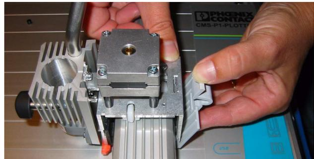
Figure 3 Attaching the counter bearing
