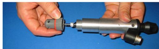
Figure 17 Unscrewing the depth adjuster
