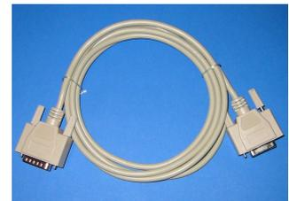
Connecting cable for control unit and plotter
