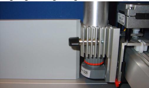
Figure 6 Alignment using the calibration block
