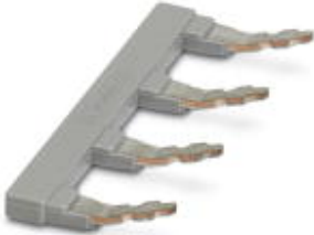
Insertion bridge, pitch: 16.4 mm, length: 24 mm, width: 55.4 mm, number of positions: 4, pin assignment: 1, 3, 5, 7, color: gray
