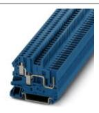
Feed-through terminal block, Connection method: Screw/plug-in connection, Cross section: 0.14 mm² - 4 mm², AWG: 26 - 12, Width: 5.2 mm, Color: blue, Mounting type: NS 35/7,5, NS 35/15
