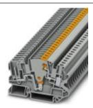
Test disconnect terminal block, Connection method: Screw/plug-in connection, Cross section: 0.14 mm² - 6 mm², AWG: 26 - 10, Width: 6.2 mm, Color: gray, Mounting type: NS 35/7,5, NS 35/15
