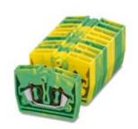
Feed-through terminal block, Connection method: Spring-cage connection, Cross section: 0.14 mm² - 2.5 mm², AWG: 26 - 14, Width: 5.2 mm, Height: 9.9 mm, Color: green-yellow, Mounting type: Screw mounting
