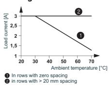
Figure shows load current depending on the ambient temperature for PLC-OSP-.../24DC/3RW. Operating time: 100% operating factor.
