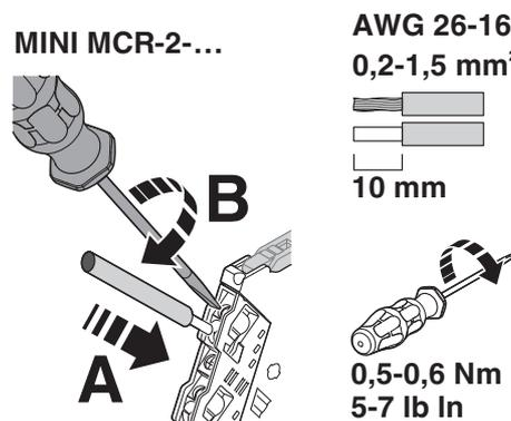
Figure 4 Screw connection
