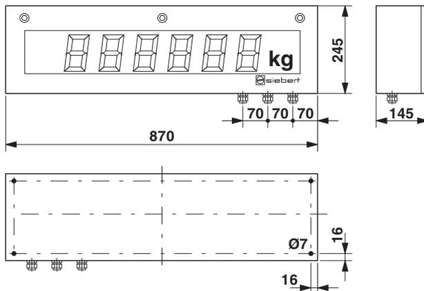
Figure 10 Dimensions of display S302 ... (dimensions in mm)
