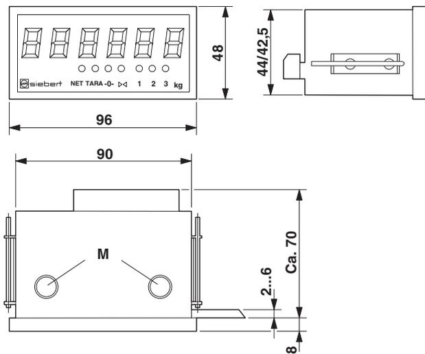
Figure 9 Dimensions of display S102 ... (dimensions in mm)
