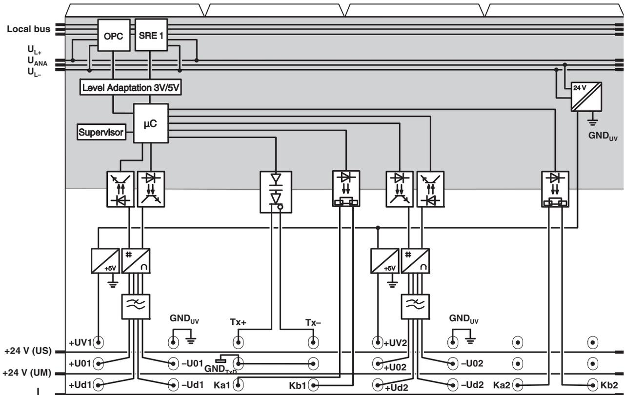
Figure 1 Internal wiring of the terminal points
