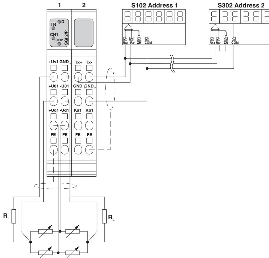
Figure 6 Connection of strain gauges in 6-wire technology
