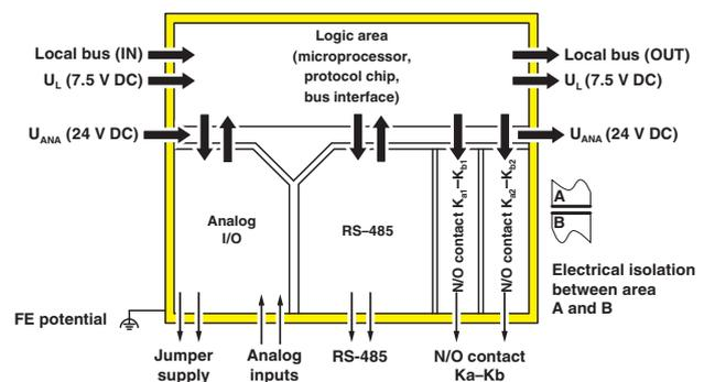
Figure 4 Electrical isolation of the individual function areas
