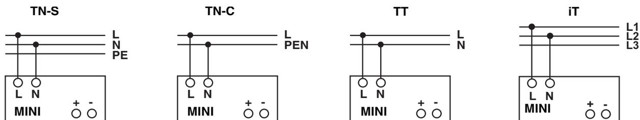
The 100...240 V AC connection is made using the L and N screw connections.
