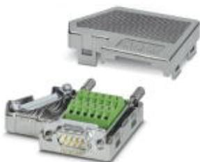
D-SUB connector, 9-pos., male connector, two cable entries < 35°, bus system: Modbus, Modbus Plus, BITBUS, ARCNET, MULT/MININET (B&R), SYSTEM 2003 (B&R), P-NET, pin assignment: 1, 2, 3, 5, 6, 8 to two screw connection terminal blocks
