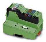
Inline XC, Bus coupler, PROFIBUS DP, D-SUB-9 female connector, Digital inputs: 8, 24 V DC, Connection method: 3-conductor, Digital outputs: 4, 24 V DC, 500 mA, Connection method: 3-conductor, Extreme conditions version, Transmission speed in the local bus 500 kBit/s / 2 MBit/s, Degree of protection IP20, including Inline connectors and marking fields
