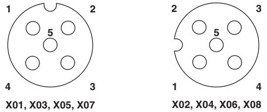
Figure 6 Pin assignment of the inputs, A-coded
