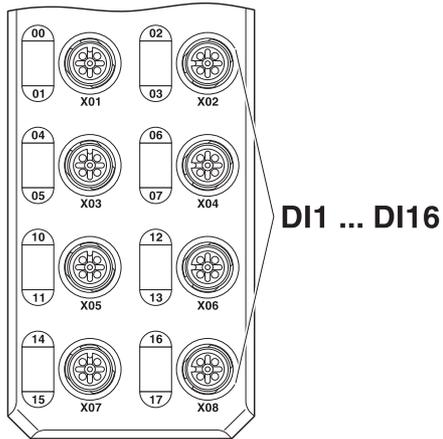
Figure 5 Input connections
