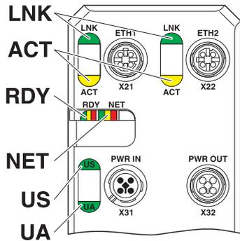
Figure 9 Indicators for Ethernet ports and power supply
