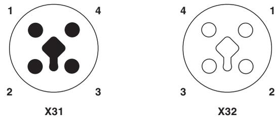
Figure 4 Pin assignment of the power supply, T-coded
