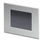
Rugged-Touch panel with 17.8 cm/7" TFT-display (Analog resistive (GFG)), 800 x 480 pixel(s) (WVGA), 16.7 million colors, Arm® Cortex®-A8, 1000 MHz, 2x USB host 2.0, 1 x Ethernet (10/100 Mbps), RJ45, Windows® Embedded Compact 7 and user software: Visu+. (bus system: without)
