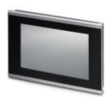
Touch panel with 22.9 cm/9" TFT-display (Projective-capacitive (PCAP)), 800 x 480 pixel(s) (WVGA), 16.7 million colors, Arm<sup>®</sup> Cortex<sup>®</sup>-A8, 1000 MHz, 2x USB host 2.0, 1 x Ethernet (10/100 Mbps), RJ45, Windows<sup>®</sup> Embedded Compact 7 and user software: Visu+. (bus system: without)
