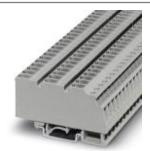
Feed-through terminal block, nom. voltage: 800 V, nominal current: 20 A, connection method: Screw/plug-in connection, number of connections: 4, number of positions: 1, cross section: 0.2 mm² - 4 mm², AWG: 24 - 12, width: 7.62 mm, color: gray, mounting type: NS 35/7,5, NS 35/15, NS 32
