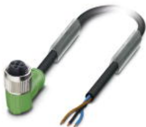
Sensor/actuator cable, 3-position, Variable cable type, free cable end, on Socket angled M12, coding: A, PIN 2+4 bridged, cable length: Free input (0.2 ... 40.0 m)
