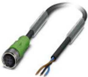
Sensor/actuator cable, 3-position, Variable cable type, free cable end, on Socket straight M12, coding: A, PIN 2+4 bridged, cable length: Free input (0.2 ... 40.0 m)
