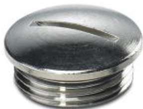
Screw plug, cable gland material: Nickel-plated brass, Brass, nickel-plated, connecting thread: Pg13.5, color: silver
