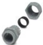
Plastic screw connection up to 5 bar, thread length: 8 mm, cable diameter: 8 - 13 mm, WAF 24, screw connection: M20
