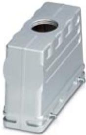
HEAVYCON sleeve housing B24, for double locking latch, height 76 mm, with thread M40, straight cable outlet, EMC version
