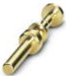
Crimp contact, turned, Single contact, Contact diameter: 3.6 mm, Crimp range: 1 mm<sup>2</sup>...2.5 mm<sup>2</sup>
