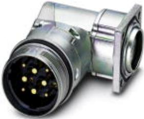
Device connector, front mounting, angled rotatable, SPEEDCON locking, M40, Number of positions: 4+3+PE, Type of contact: Male connector, Crimp connection, Axial O-ring, 4xØ4,4, Shielded: Yes, Flange dimensions: 40 mm x 40 mm
