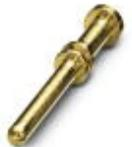
Crimp contact, turned, Single contact, Contact diameter: 2 mm, Crimp range: 0.14 mm<sup>2</sup>...0.25 mm<sup>2</sup>
