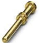
Crimp contact, turned, Single contact, Contact diameter: 2 mm, Crimp range: 0.25 mm<sup>2</sup>...1 mm<sup>2</sup>
