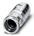
Sleeve housing for coupler connector, straight, Bayonet locking, M23, shielded: yes, cable diameter range: 2 mm 14.5 mm
