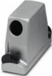
HEAVYCON ADVANCE EMV sleeve housing B24, with bayonet locking, height 100 mm, with 1xM40 thread, lateral cable outlet
